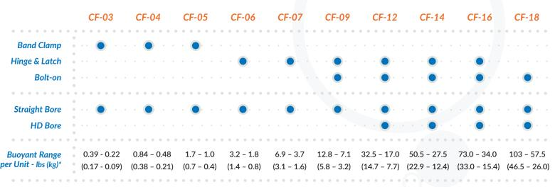
\*Buoyant range based on average nominal buoyancy achieved per unit from our most shallow rated material (750m) to our deepest rated material (6000m)
