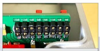
A text opposite to the jumpers shows where the pair of jumpers should be placed to get wanted output gain.
