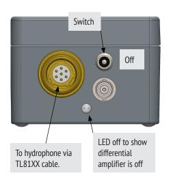
Differential output of hydrophone on the XLR connector
