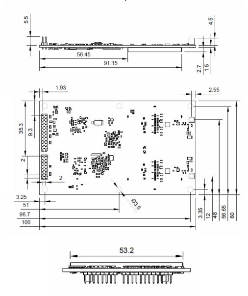
Figure 2-1: Vega 40 mechanical layout
