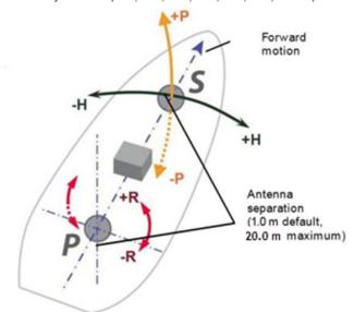
Figure 3-5: Recommended orientation and resulting signs of HPR values
