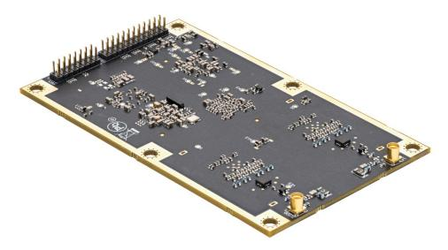
Figure 1-1: Vega 40 GNSS OEM board
