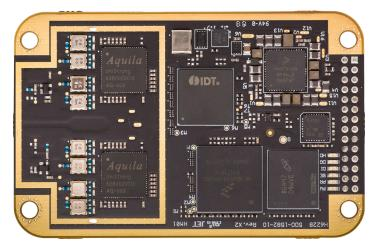
The Vega 28 is our most advanced GNSS heading and positioning board.
