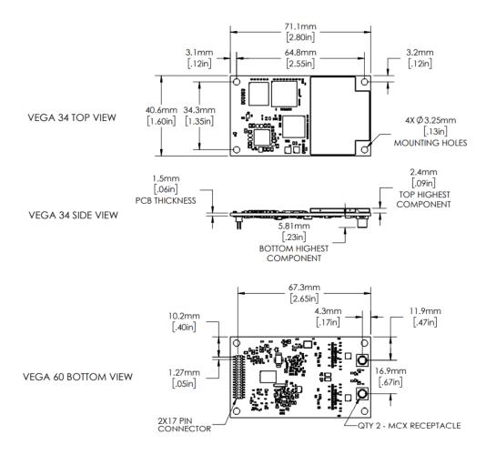
Figure 2-2: Vega 34 mechanical layout
