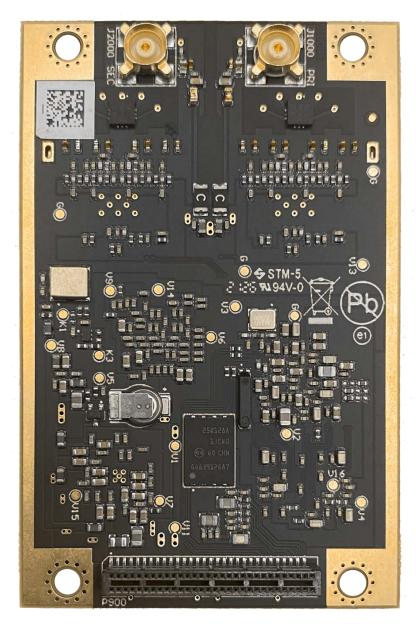
Figure 1-3: Vega 60 GNSS OEM Board
