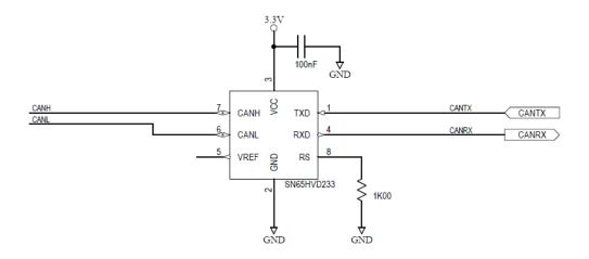
Figure 2-8: Vega 28 CAN design example
