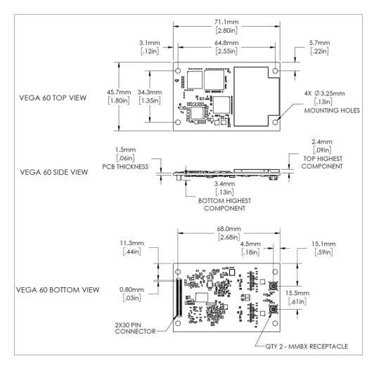
Figure 2-3: Vega 60 mechanical layout
