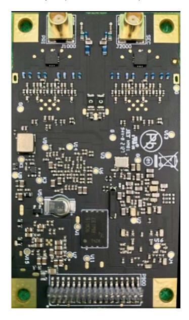
Figure 1-2: Vega 34 GNSS OEM Board
