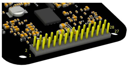
Figure 2-5: Vega 28 pin layout
