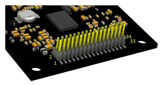
Figure 2-6: Vega 34 - 34-pin header layout
