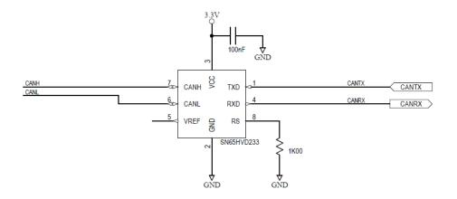
Figure 2-10: Vega 60 CAN design example
