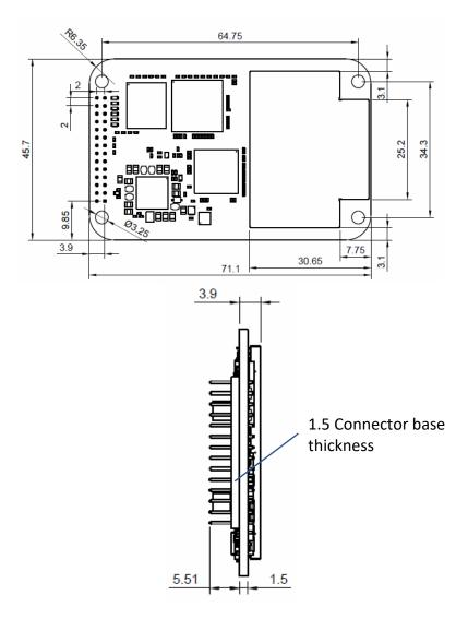
Figure 2-1: Vega 28 mechanical layout
