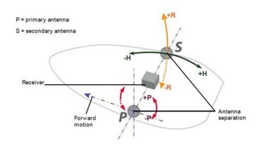
Figure 3-6: Alternate orientation and resulting signs of HPR values
