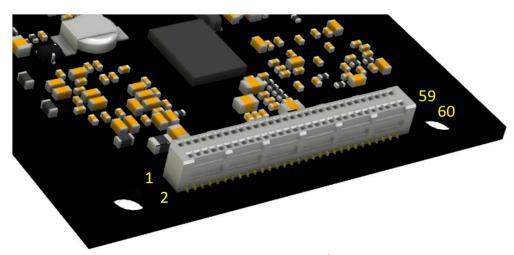
Figure 2-7: Vega 60 60-pin layout
