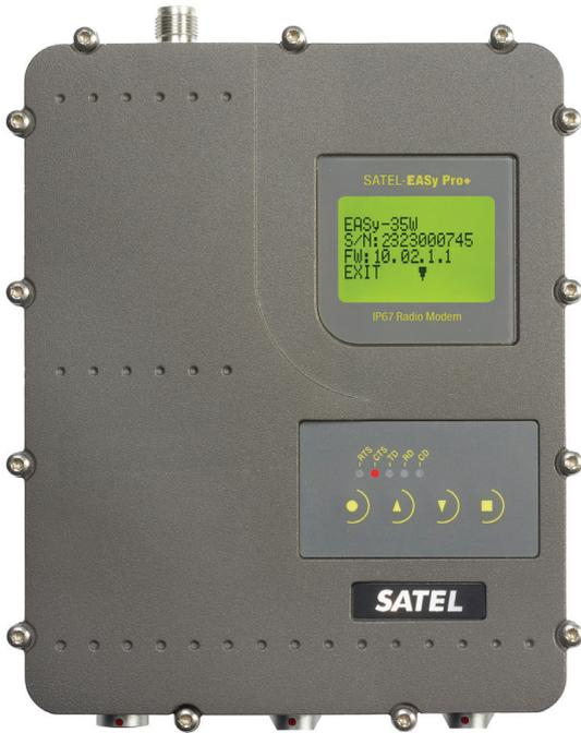
SATEL-EASy Pro+ is a new IP67 classified UHF radio modem from SATEL product portfolio. It comes with a high power up to 35 W transmitter and wide 70 MHz tuning range.
