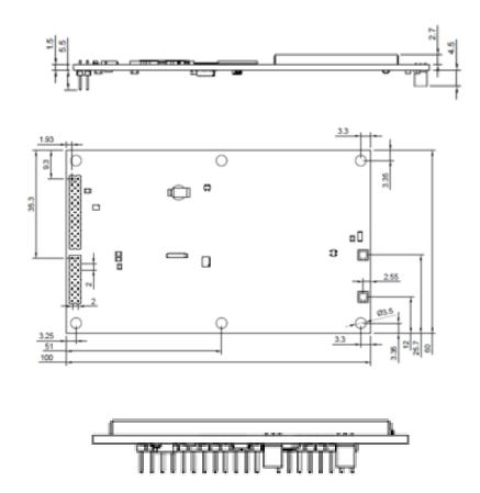
Figure 2-1: Phantom 40 mechanical layout
