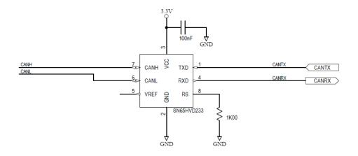
Figure 2-5: Phantom 40 CAN design example
