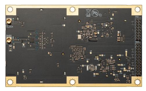
Figure 1-1: Phantom 40 GNSS OEM Board
