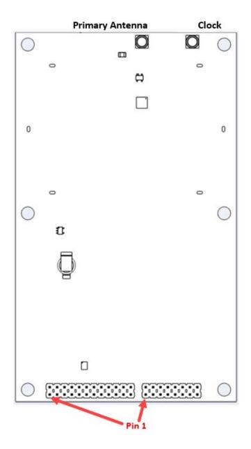
Figure 2-2: Phantom 40 Connectors
