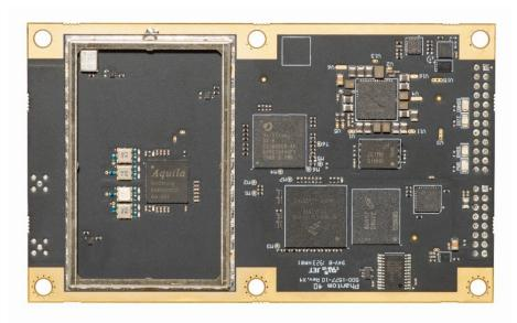
Figure 1-2: Phantom 40 GNSS OEM Board
