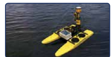
HyDrone™ ASV with Trimble SPS 585 and TSC3
