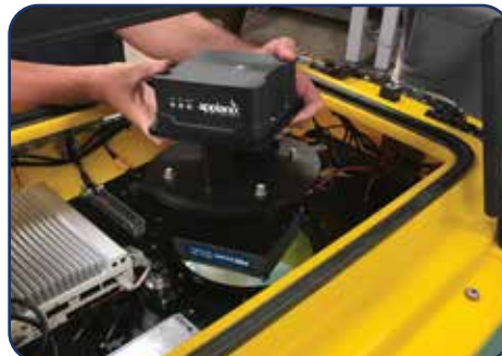
R2 Sonic MultiBeam, Applanix POS MV Surfmaster
