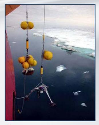
The 8242XS Acoustic Release Transponder is a field-proven, reliable, and versatile mooring instrument. The 8242XS is made entirely of Nickel Aluminum Bronze alloy with titanium closure hardware for very long deployments with no corrosion. Acoustic status reply includes tilt and release state. Command structure proven in the toughest acoustic environments anywhere. Many of these releases are over 15 years old and still in use.
