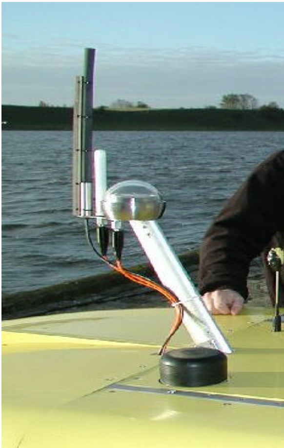
Figure 3 : GPS antenna mounted on MARIDAN AUV M600
